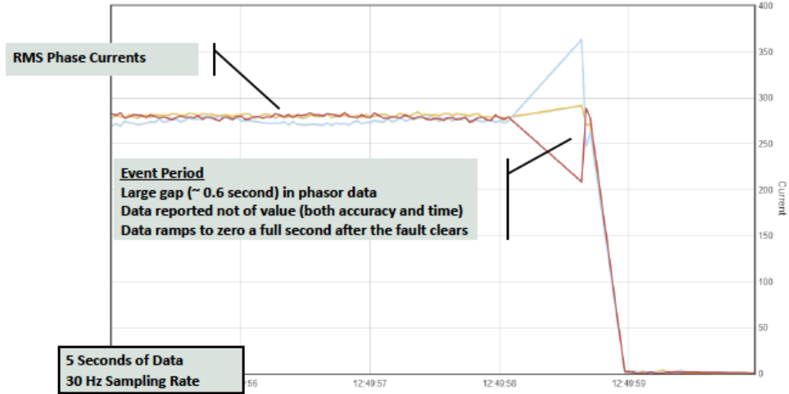
Based on synchrophasor data collected by TVA's openPDC from a PMU
