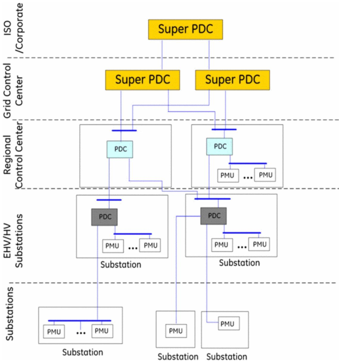
**Figure 18: Wide Area Measurement System (WAMS) hierarchy [13]**
