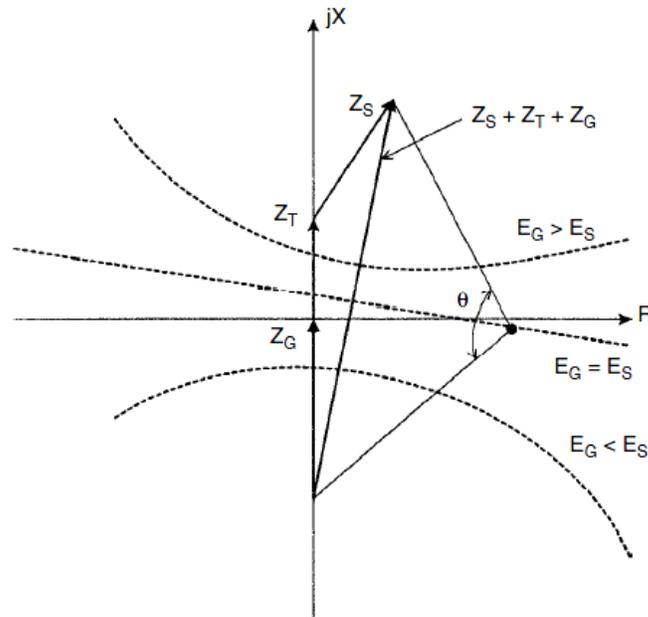
**Figure 9: Impedance trajectory during a power swing [1]**
