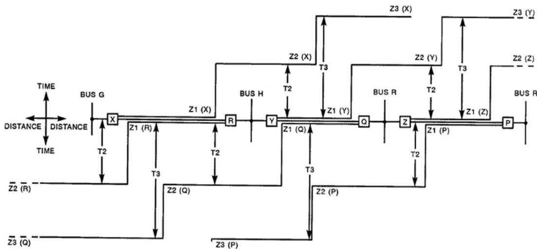
**Figure 5: Step Distance Zone protection**
