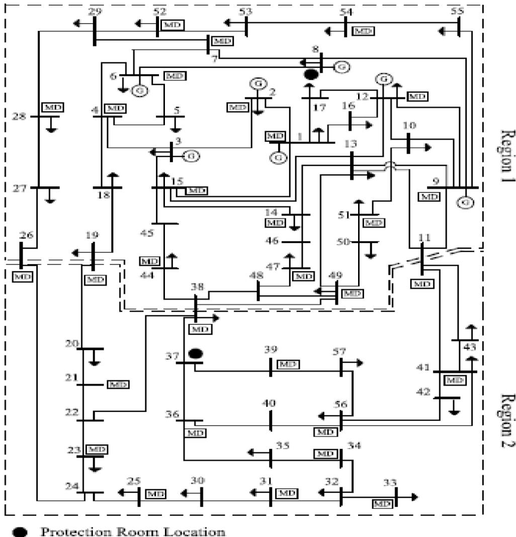
**Figure 19: IEEE 57-bus test system. MDs and protection room location and specified protection regions [14]**
