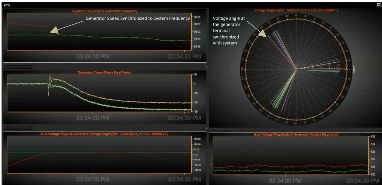
**Figure 17b: Synchronization of Post-Synchronization of Large Coal Unit in Dominion System**
