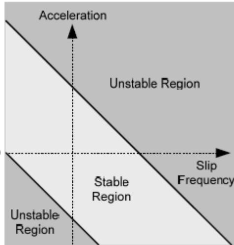
**Figure 7: Out of Step stability graph**
