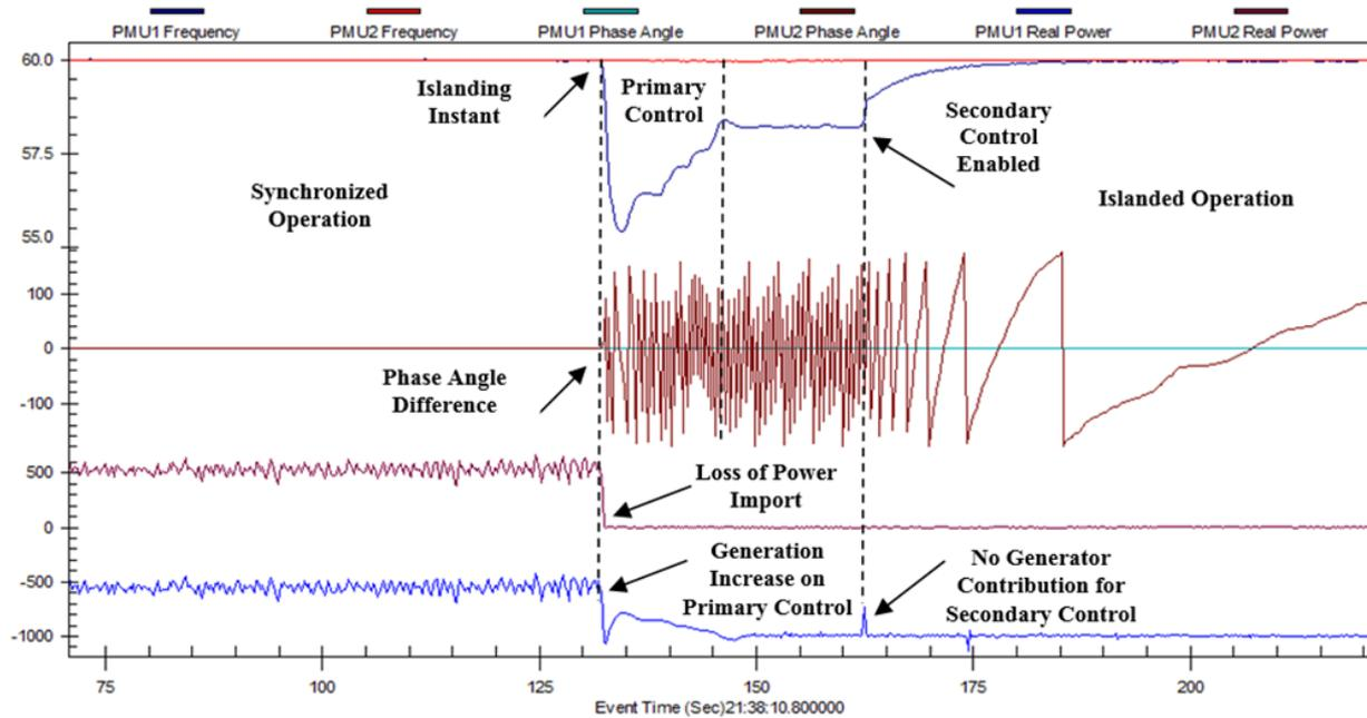
**Figure 14: Simulation of Islanding and Microgrid Controls**
