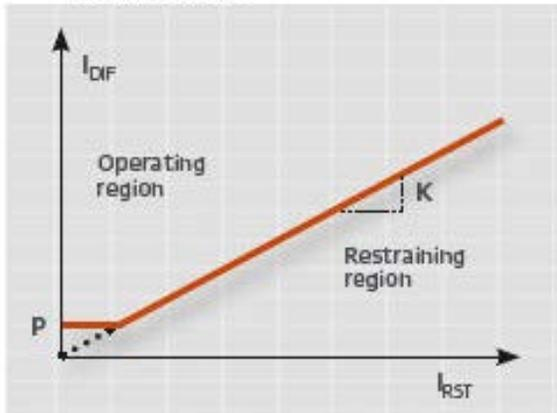
b) Fictitious differential signal due to CT errors & dual-slope percentage differential characteristics
