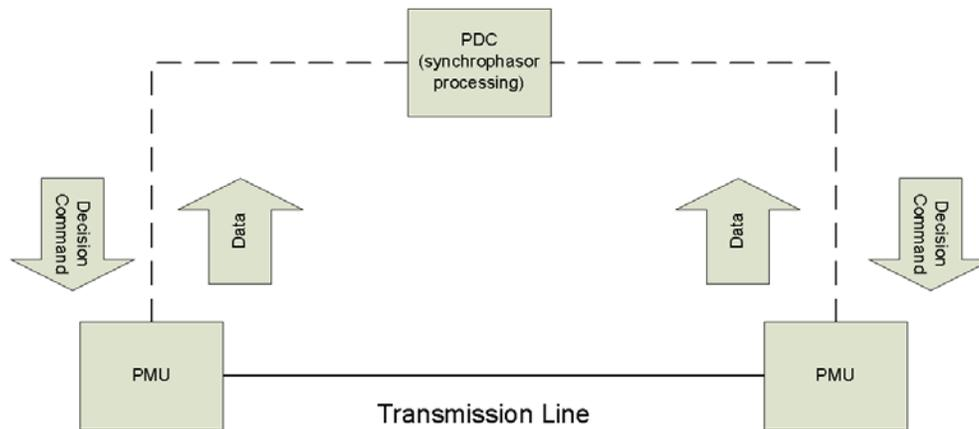
**Figure 2: PMU to PDC to PMU Network Architecture**
