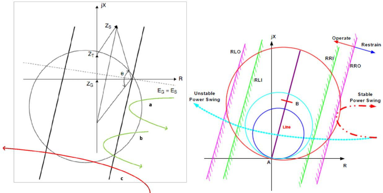
**Figure 10: Single and double blinder out-of-step protection schemes [2]**
