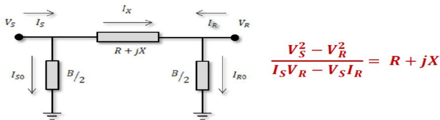
**Figure 11: Transmission Line Circuit and Impedance Calculation [10]**
