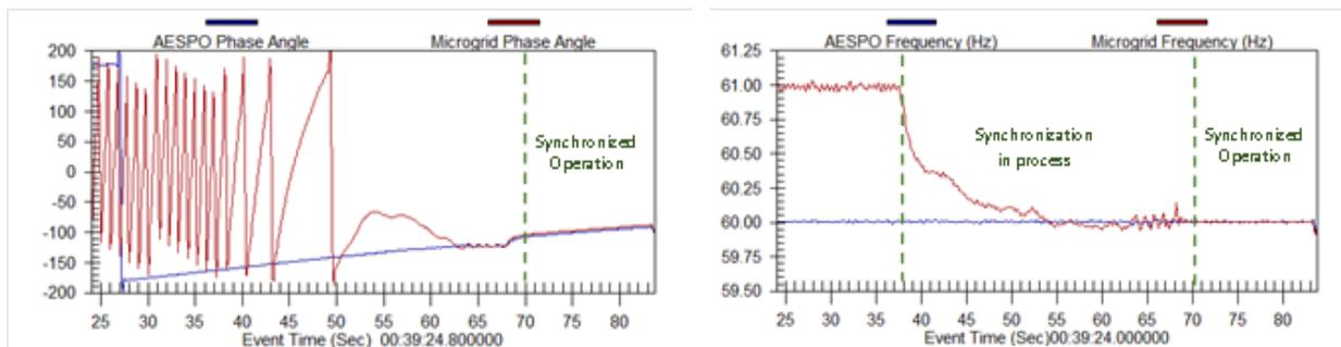
**Figure 15: Resynchronization of the Microgrid**
