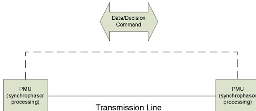
**Figure 1: PMU to PMU Network Architecture**
