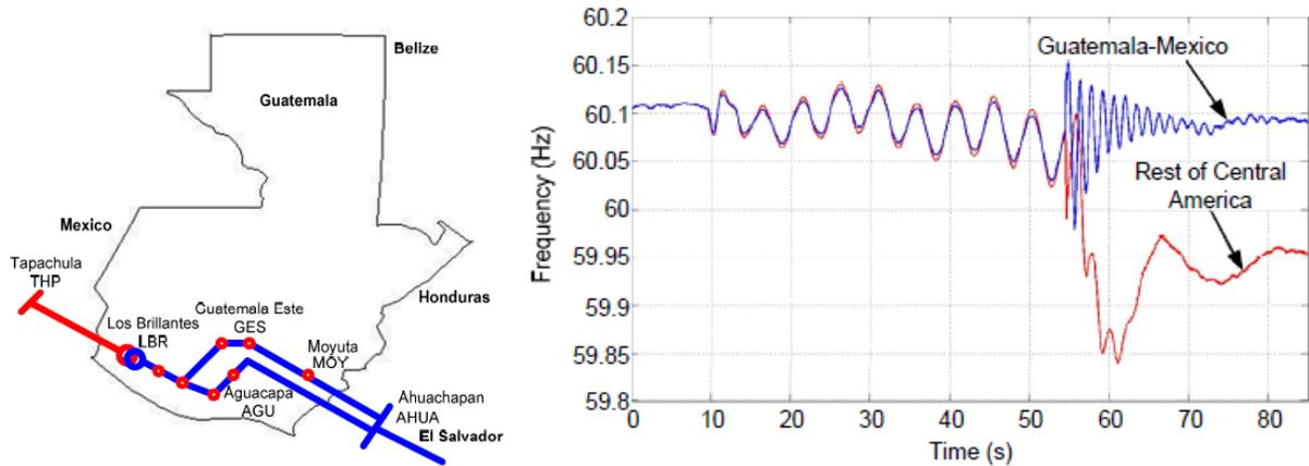
**Figure 12: Guatemalan Power System and PMU-Based Stability Scheme [8]**
