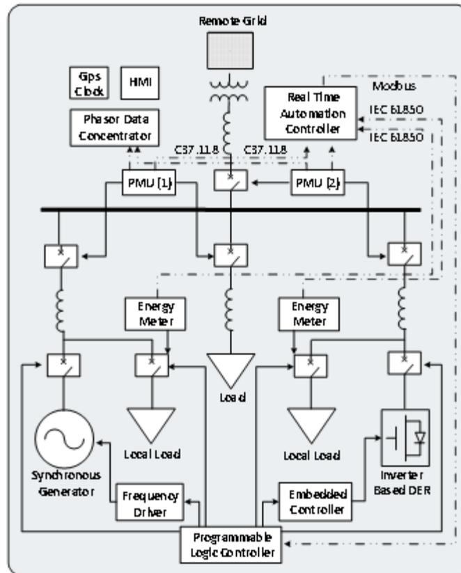
**Figure 13: Microgrid Architecture [9]**
