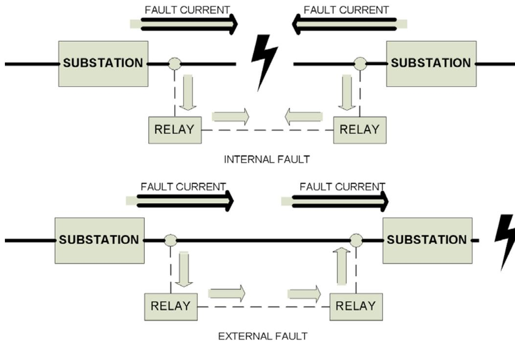
**Figure 6: Transmission Line Differential Protection Theory of Operation**
