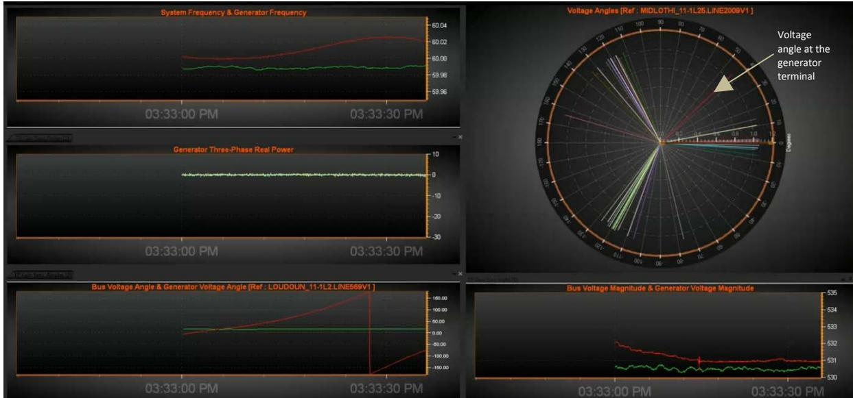
**Figure 17a: Synchrophasor data pre-synchronization of large coal unit in Dominion system**
