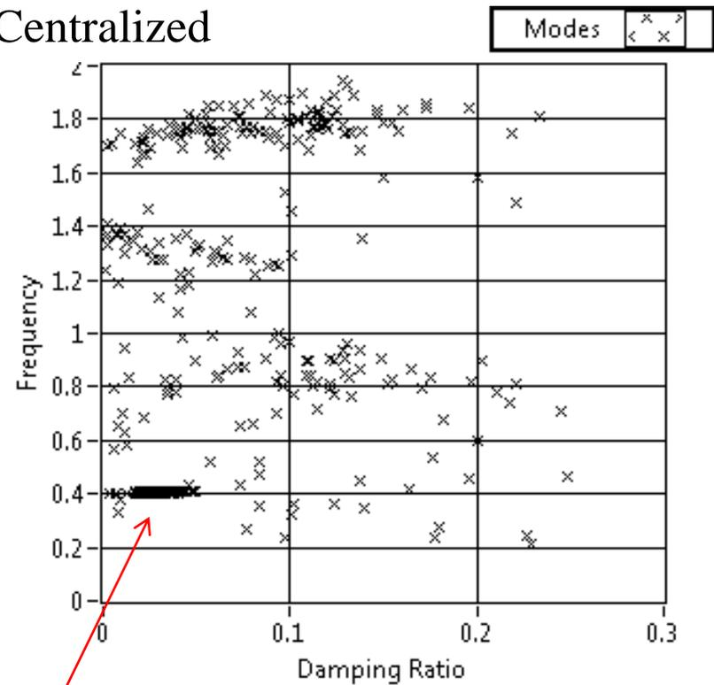
Inter-area oscillatory mode between HV section and rest of the grid
