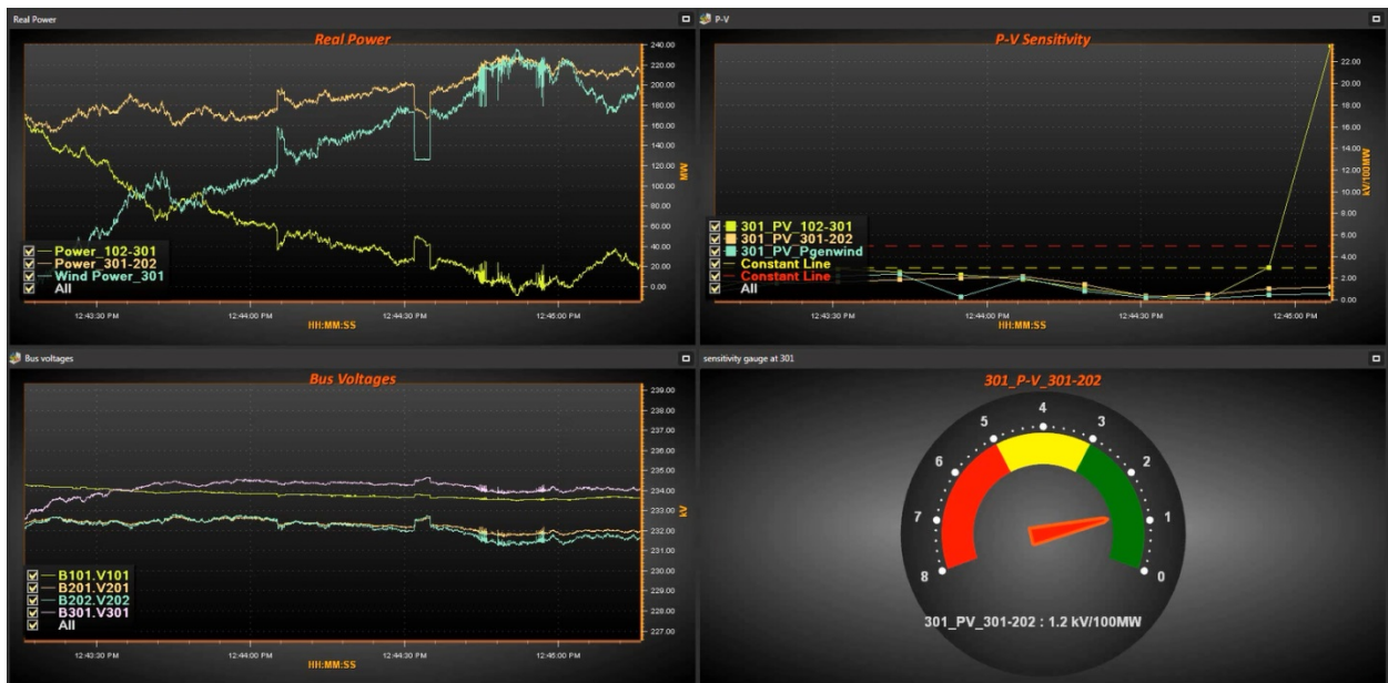
Fig. 4. Left two charts: Voltage and power flow line charts of monitored locations; Top right: Sensitivity trend chart showing history with alarm threshold; Bottom right: Sensitivity gauge showing current sensitivity value with alarm threshold
