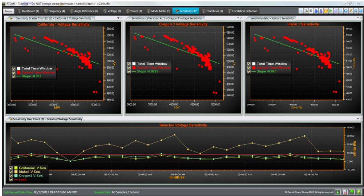
Fig. 3. Top: Sensitivity scatter chart for different locations being monitored; Bottom: Sensitivity trend chart showing history with alarm threshold
