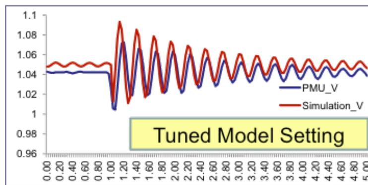
**Figure 39. ERCOT's PMU-tuned dynamic wind plant model**
