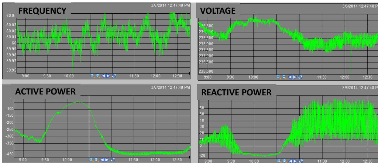
Example 2 – Another wind plant ramp causing oscillations
