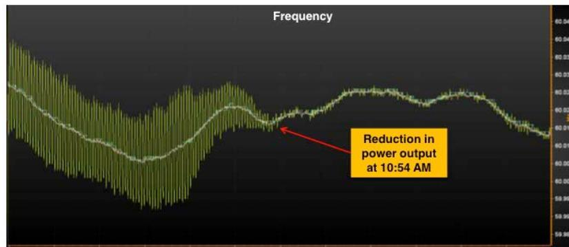
**Figure 35. Oscillations stopped after wind plant power output dropped from 45 to 40 MW**
