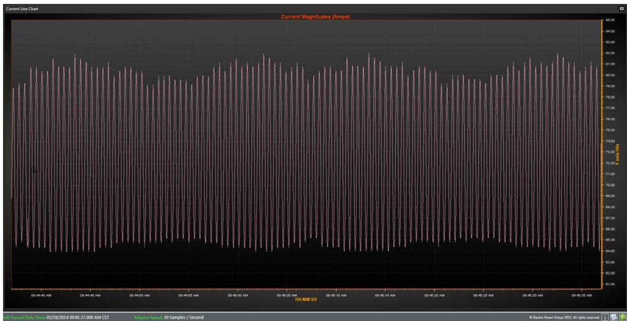
**Figure 22. Current oscillations on West 4 PM**
