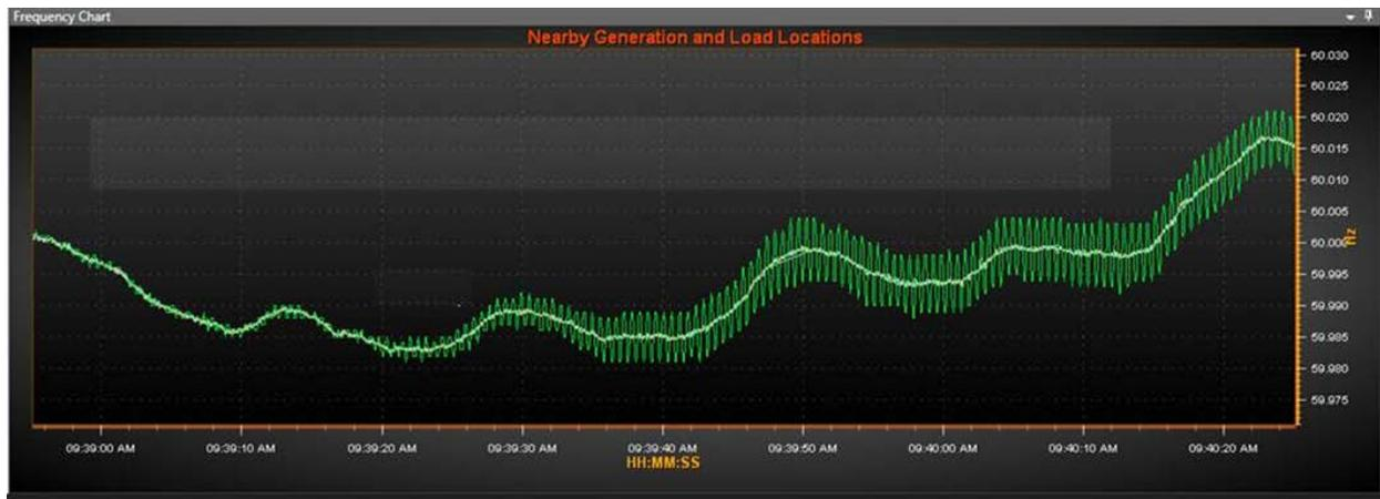
**Figure 21. Frequency oscillation on West 4 PM**
