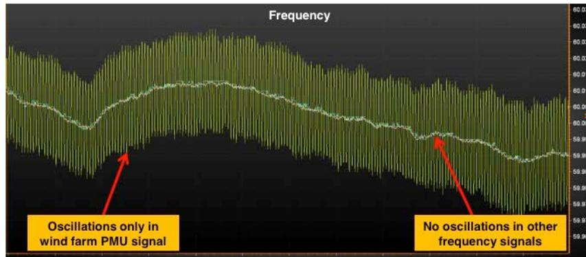
**Figure 33. Continuing oscillations on Day 2 for a total of 17 hours**
