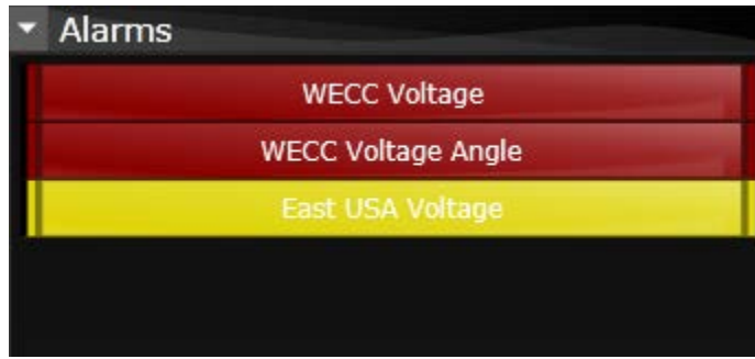
Figure 16: Alarm Panel Display in SEL's SynchroWAVE Tool
