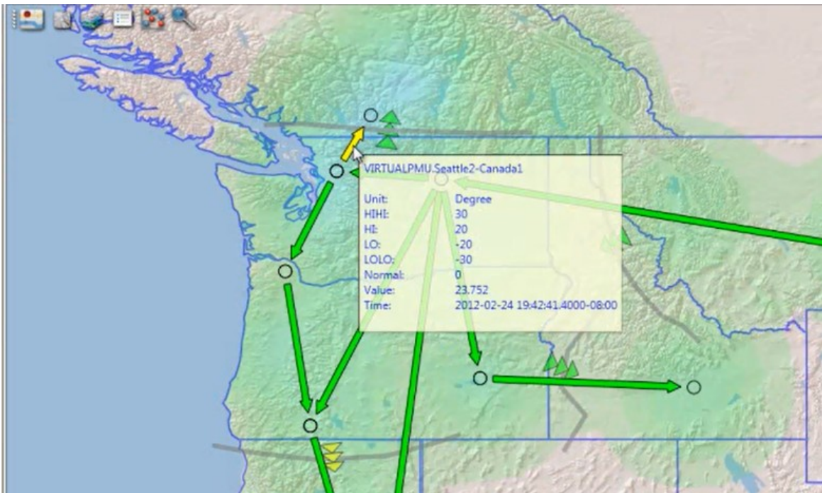
Figure 13: Typical dashboard with phase angle difference layer in map in EPG's RTDMS Tool. Corresponding alarm shows in alarm panel on the right.
