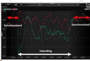
Frequency of the two system when in synchronization and when separated from each other.
