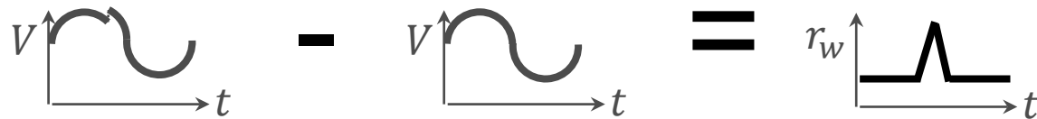
Minimum detectable Temporary Voltage drop (1.2% reduction)
