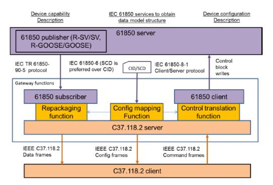
Use case-A: Data, Configuration and Command exchange
