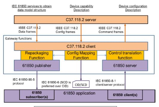
Use case-B: Data, Configuration, and Command exchange
