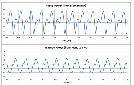
Multiple instances of oscillations were detected at a hydro-power under light load conditions
