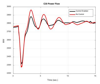
System test performed with modulation controller enabled and controller off
