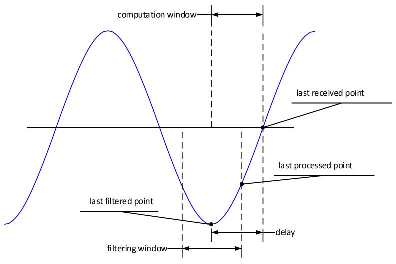
Computation window – 10 ms, filtering window – 5 ms
