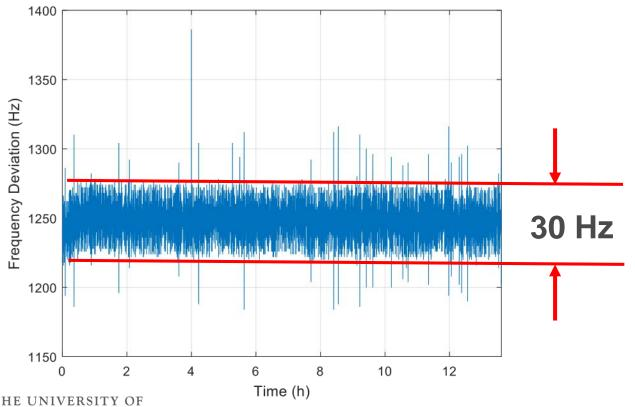
Test of a 40 MHz Oscillator inside PMU
