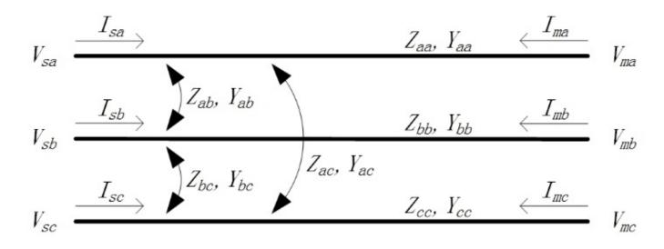
Assume PMU measurements at both terminals of the line.
