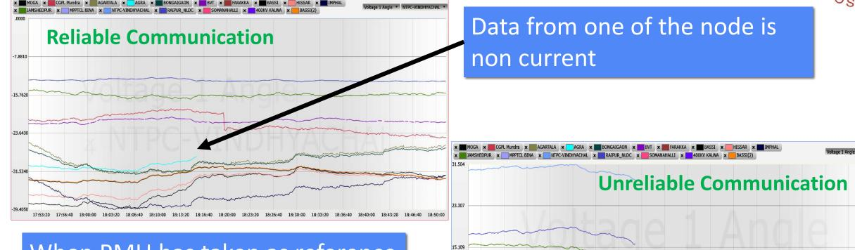
When PMU has taken as reference whose data is not updating, Rest of Angular Separation can not be visualized
