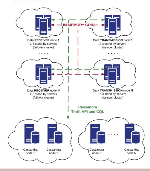
Provides real-time data collection from various sources (PMU, RTU – SCADA, DFR and other IEDs) with high performance (hundreds thousands of measurements per second), scalability and fault-tolerance and distributed nodes cluster capabilities.
