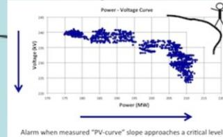
Alarm when measured "PV-curve" slope approaches a critical level
