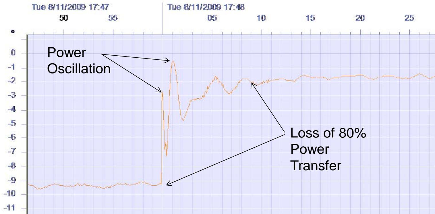
$$P = V_1 V_2 \sin \Theta / X$$
