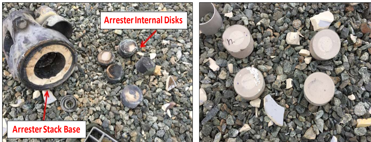
Internal MOV Disks from C-phase (left) and A-phase (right) Arresters
