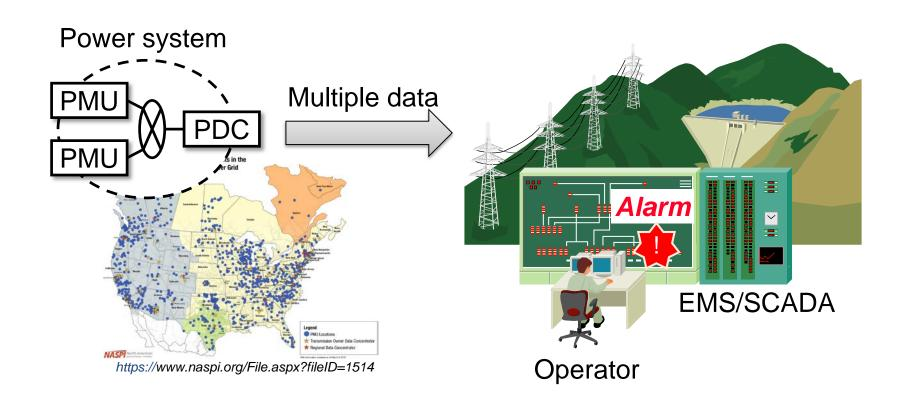
PMU: Phasor Measurement Unit, SCADA: Supervisory Control and Data Acquisition,
