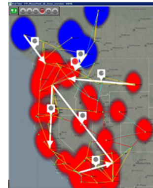
Figure 9: Geospatial displays showing angle difference monitoring in ALSTOM Grid Tool.
