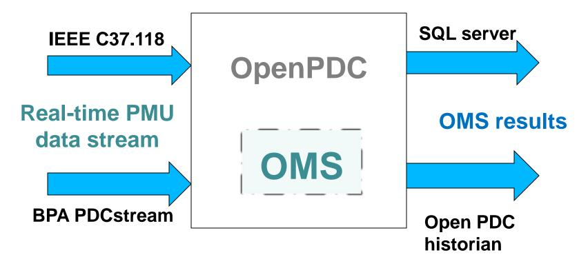
OMS action adapter built into OpenPDC 64 bit version 2.1.
