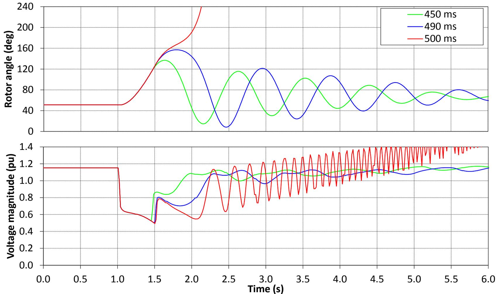
Variations of rotor angle and voltage magnitude following a fault
