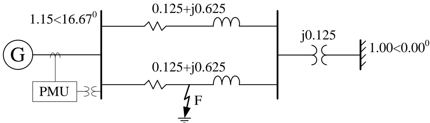
One machine to infinite bus (OMIB) system with the initial steady-state power flow solution
