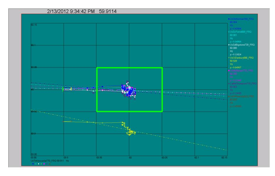
• X-Y plot of 7 frequencies in the Eastern Interconnection versus Knoxville frequency
