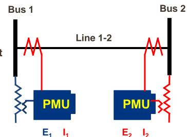
PMUs at two ends of the line provide 4 sets of measurements:  $E_1$ ,  $E_2$ ,  $I_1$ , and  $I_2$ . Using multiple sets of these measurements obtained over several hours of system load variations the unknown RCFs can be determined.
