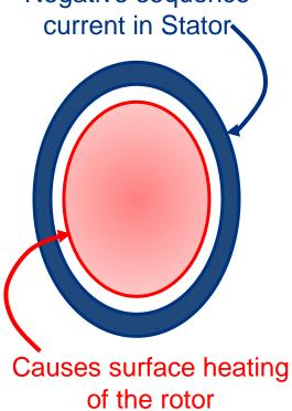
Negative sequence currents are continuously monitored on the network. Summing up all negative sequence currents in lines connected to generators, the generator negative sequence currents can be monitored.
