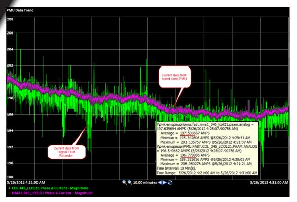
DFRs built to display data for faults (thousands of amps) which impacts how things look when operating in the 0 to 100 amp range
