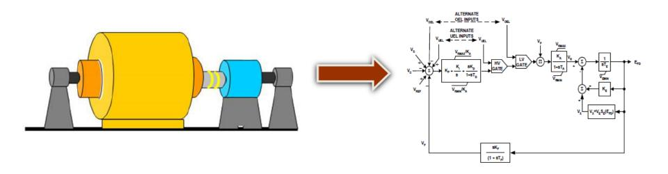
Challenge: Build a good dynamic model for a Generator/Excitation System that matches the actual equipment in the field and validate it through offline/online testing
