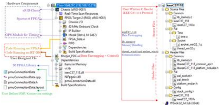
Code structure for Synchrophasor Synchronization Gateway + Controller on cRIO-9081
