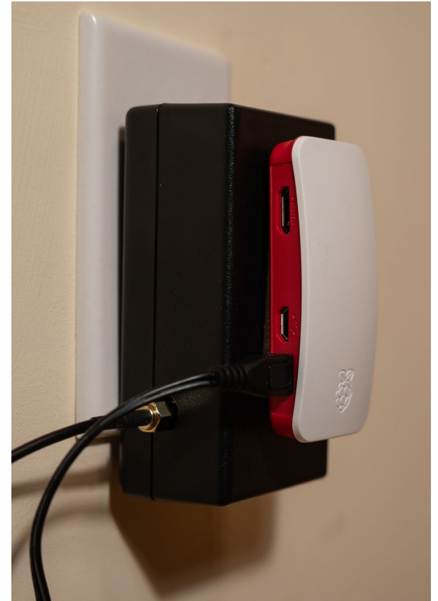
32 ksps “Archiver” deployment with GPS and 1.5 TB of storage on Raspberry Pi Zero 2W
