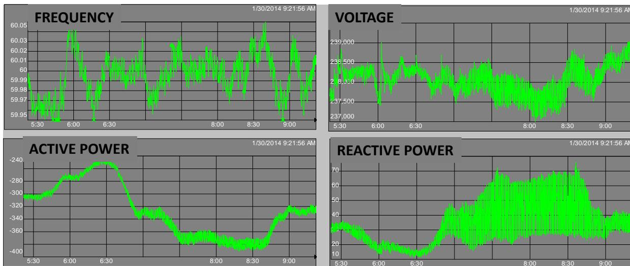
Example 1 – Wind generation ramp with high oscillations before control upgrade
