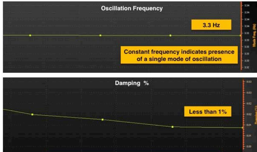
**Figure 34. Constant oscillation frequency and low damping coefficient for the duration of the oscillations**
