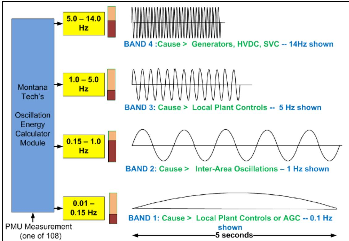
Example based on Montana Tech Oscillation Energy Calculator
