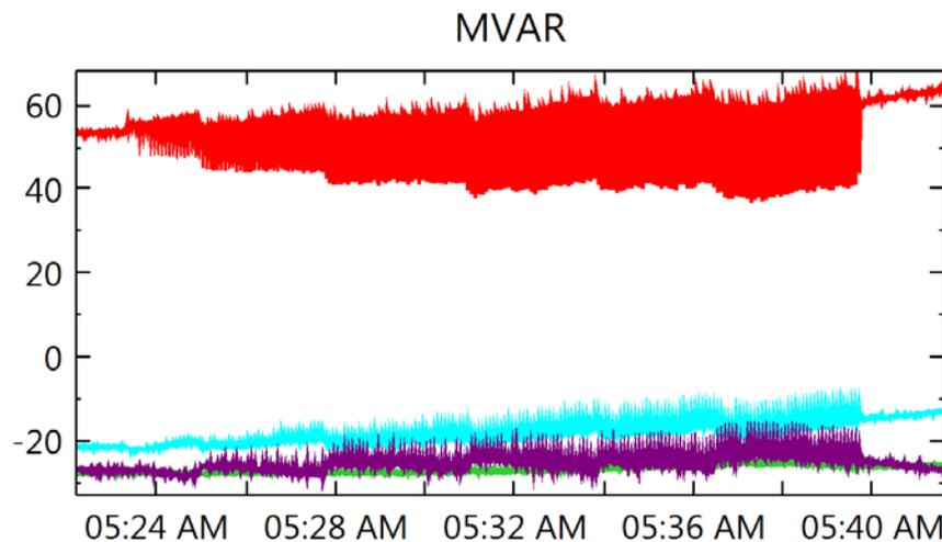
**Figure 9. Reactive power (MVAR) oscillations on one unit of four generators**
