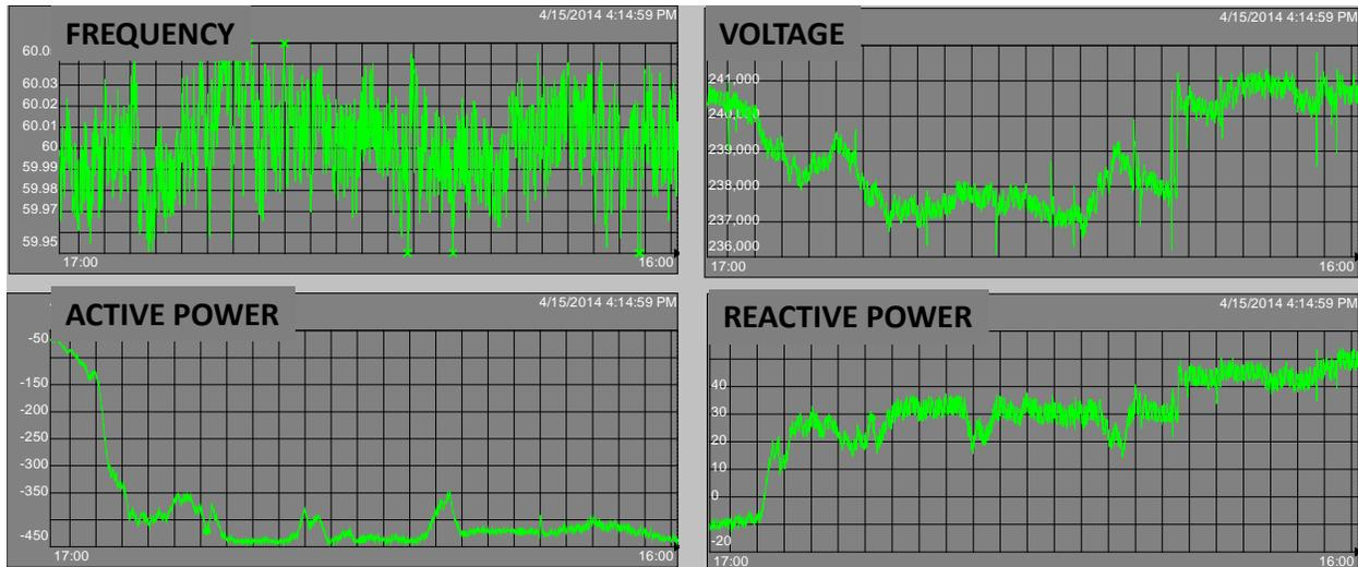
Example 3 – Wind generation ramp after control upgrade, with lower magnitude of oscillations
