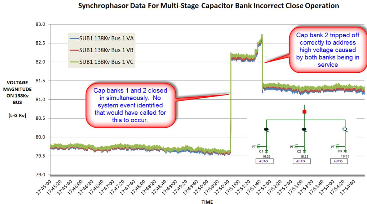
**Figure 52. Capacitor bank switching problem at ATC**
