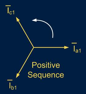
Balanced  $\overline{I}_{b1} = a^2 \overline{I}_{a1}$   $\overline{I}_{c1} = a \overline{I}_{a1}$
