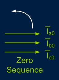
Single Phase  $\overline{I}_{a0} = \overline{I}_{b0} = \overline{I}_{c0}$
