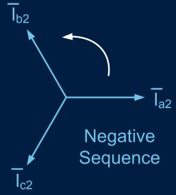
Balanced  $\overline{I}_{b2} = \overline{aI}_{a2}$   $\overline{I}_{c2} = \overline{a^2I}_{a2}$
