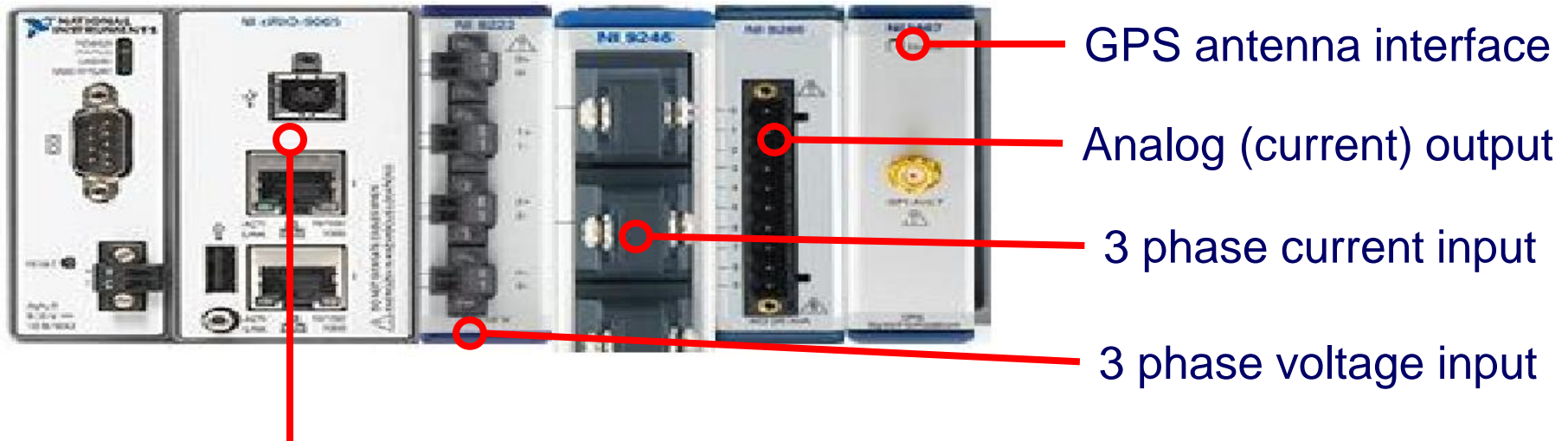
Compact Reconfigurable I/O (FPGA + microprocessor hardware) with TCP/IP communication
