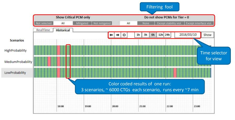
Color coding of PCMs: Acceptable; Near critical; Critical; Voltage collapse which could be
