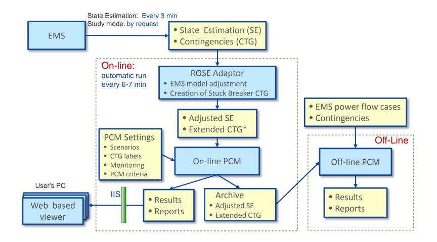
\* Extended CTG include selected N-2 used in Day-Ahead processes and all Stuck Breaker. Total ~6,000 x 3 = 18,000 CTGs
