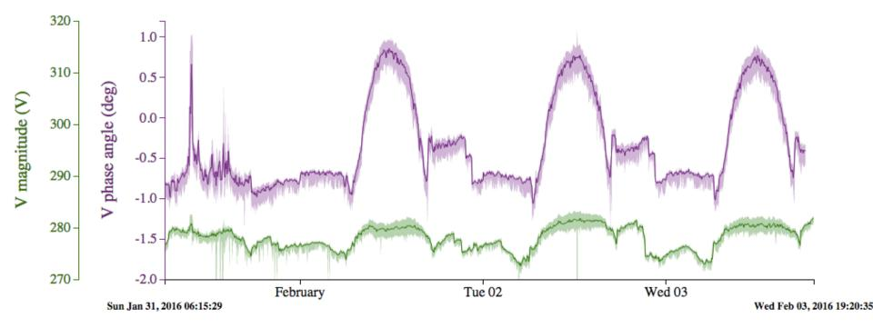
µPMU Measurements on a distribution feeder with high-penetration PV, illustrating relationship between voltage phase angle difference and power flow
